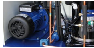
Pump P3 (3 barg) / P5 pump (5 barg, optional).
